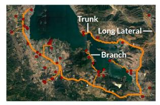
Adding measurements of all the fiber elements and applying an industry benchmark for rural trenching costs per mile yields a total cost for the trenching in this project of \$6.8M, or \$120k per location. Trenching alone for the all-fiber approach is more than 40x the cost of the complete DigitalPath deployment.
